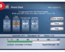
Once accurately pointed, the signal meter will turn green. Make small adjustments to get the signal as high as possible. Check that the bar at the bottom of
